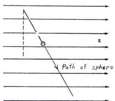
After the string is cut, the only forces are gravity, which acts down, and the electrical force, which acts to the right.
