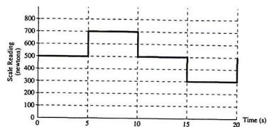
1993B1. A student whose normal weight is 500 newtons stands on a scale in an elevator and records the scale reading as a function of time. The data are shown in the graph above. At time t = 0, the elevator is at displacement x = 0 with velocity v = 0. Assume that the positive directions for displacement, velocity, and acceleration are upward.
