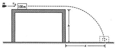
1990B1. A bullet of mass m is moving horizontally with speed  $v_o$  when it hits a block of mass 100m that is at rest on a horizontal frictionless table, as shown above. The surface of the table is a height h above the floor. After the impact the bullet and the block slide off the table and hit the floor a distance x from the edge of the table. Derive expressions for the following quantities in terms of m, h,  $v_o$ , and appropriate constants:
