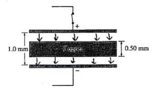
iv. E = V/d and you can use the entire gap or just one of the two gaps; E = 30 V/(0.5 mm) or 15 V/(0.25 mm) E = 60 V/mm or 60,000 V/m
