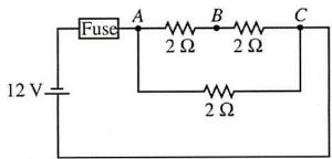
An electric circuit consists of a 12 V battery, an ideal 10 A fuse, and three 2 Ω resistors connected as shown above.
