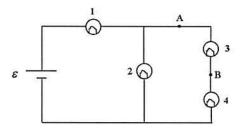
118. For the circuit shown, a shorting wire of negligible resistance is added to the circuit between points A and B. When this shorting wire is added, bulb #3 goes out. Which bulbs (all identical) in the circuit brighten?
