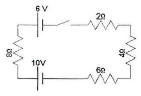
141. When the switch is closed, what would be the current in the circuit shown in the diagram above if the two batteries are opposing one another?
