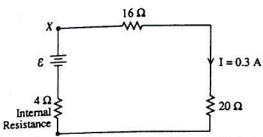
The above circuit diagram shows a battery with an internal resistance of 4.0 ohms connected to a 16-ohm and a 20-ohm resistor in series. The current in the 20-ohm resistor is 0.3 amperes
