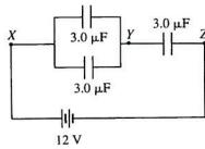
Three identical capacitors, each of capacitance 3.0 µF, are connected in a circuit with a 12 V battery as shown above.
