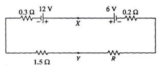
In the circuit above, the emf's and the resistances have the values shown. The current I in the circuit is 2 amperes.
