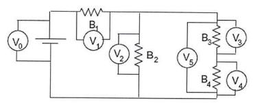
$B_1, B_2, B_3$ , and  $B_4$  are identical light bulbs. There are six voltmeters connected to the circuit as shown. All voltmeters are connected so that they display positive voltages. Assume that the voltmeters do not affect the circuit.
