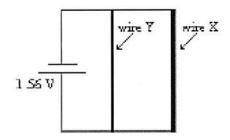
96. The following diagram represents an electrical circuit containing two uniform resistance wires connected to a single flashlight cell. Both wires have the same length, but the thickness of wire X is twice that of wire Y. Which of the following would best represent the dependence of electric potential on position along the length of the two wires?
