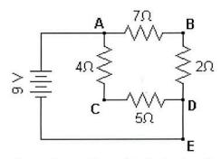
A 9-volt battery is connected to four resistors to form a simple circuit as shown above.
