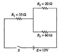
72. In the circuit shown above, the equivalent resistance of the three resistors is (A)  $10.5 \Omega$  (B)  $15\Omega$  (C)  $20 \Omega$  (D)  $50 \Omega$  (E)  $115 \Omega$
